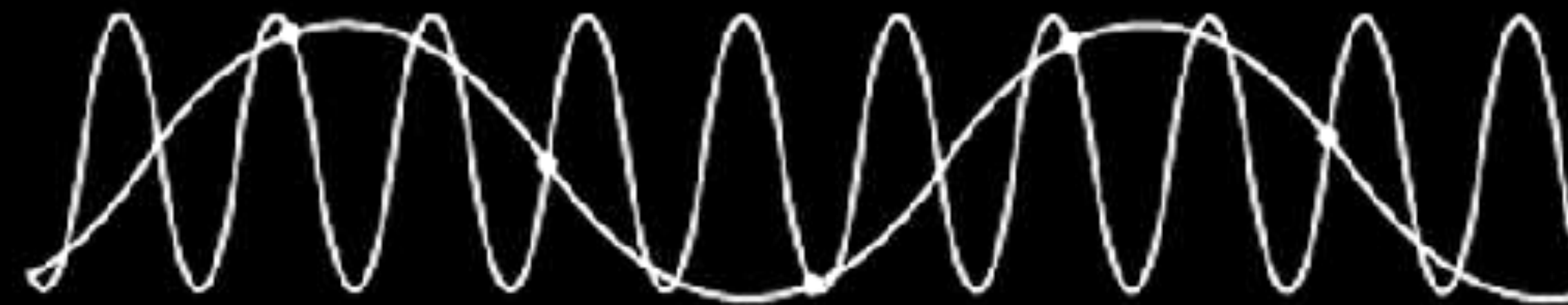
Aliased Signal Due to Undersampling
